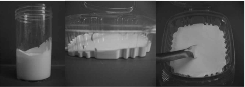
Figure 8. Pictures of the obtained cross-flow filtration retentate; 1.8 wt% DV834; 68.9 wt% dryness.
